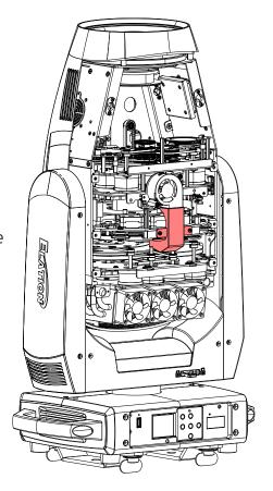
Locate the Gobo Module, remove the screws that secure it to the internal housing frame, and unplug/disconnect wire harness.
