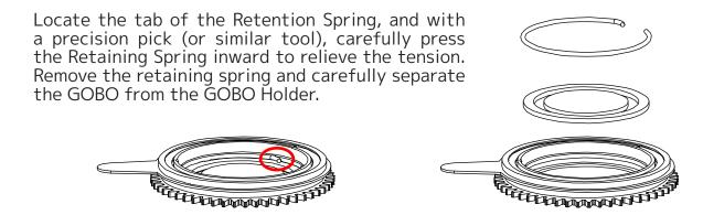
**Note**: To ensure proper Gobo orientation on the Rotating Gobo Wheel, align the Alignment Indices before installing the Retention Spring.
