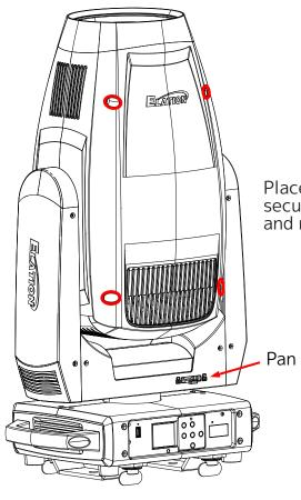
Place the fixture on a firm flat surface. Locate the (4x) screws securing the panel on the **Pan Lock** side of the moving head and remove them.
