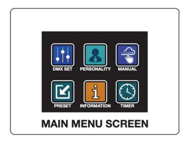
To proceed, press the main menu icon that you would like to access. Use the **ENTER** button to access sub menus and use the **UP** and **DOWN** buttons to make adjustments. Press the **ENTER** button to confirm your adjustments. You may exit the main menu at any time without making any adjustments by pressing the **BACK/EXIT** button.
