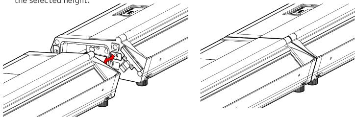
With the heights of adjacent fixtures adjusted to a matching height, orient the alignment features and move them together to allow their magnets to connect them and maintain their relative positions.
