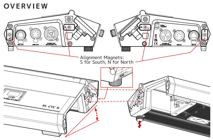
The corollary alignment features of the fixture, magnets, projections, and cavities, are designed to interlock when placed adjacent to each other with the same orientation. The front of the fixture can be raised or lowered to match these interlocking features, or to adjust the projection height of the fixture.
