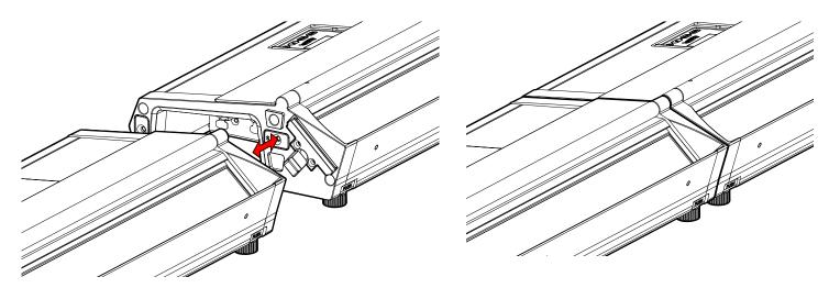
With the heights of adjacent fixtures adjusted to a matching height, orient the alignment features and move them together to allow their magnets to connect them and maintain their relative positions.
