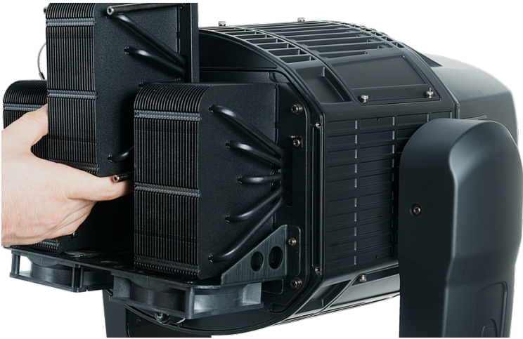
6. Unclip the center heatsink module safety cable.
