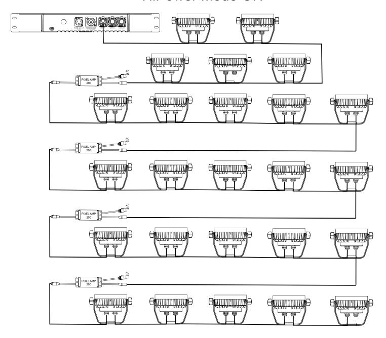
For all drivers, with HiPower Mode OFF, each port can drive a maximum of 8(x) Elation Pixel Wash 40IP fixtures, or a maximum of 40(x) fixtures when incorporating up to 4(x) Pixel Amp 200's (sold separately) as shown below.
