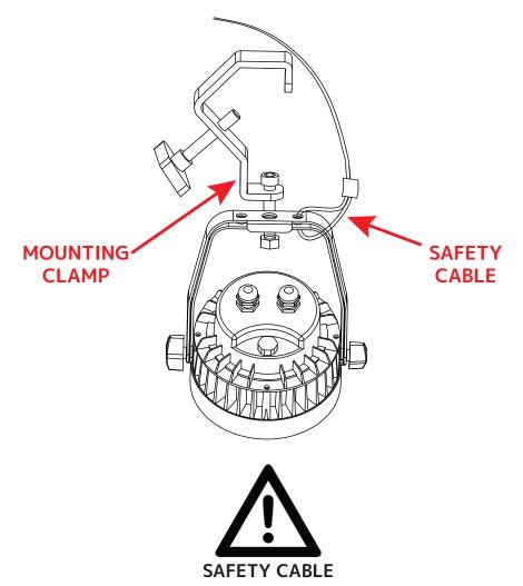
ALWAYS ATTACH A SAFETY CABLE WHENEVER INSTALLING THIS FIXTURE IN A SUSPENDED ENVIRONMENT TO ENSURE THAT THE FIXTURE WILL NOT FALL IF THE CLAMP FAILS.
