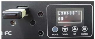
Use the **UP** and **DOWN** buttons to select software, and press **ENTER**, then select **ON**, and press **ENTER**, at which time the software will begin loading.
