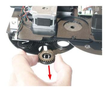
7. Locate the rotating gobo that will be replaced. Grip the edges of the geared gobo holder and gently lift (pictured at left) until the gobo holder clears the surface of the gobo wheel. Then pull the gobo holder out and away (pictured at right).
