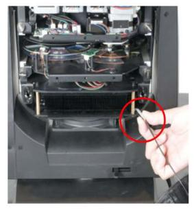
2. Use a Phillips head screwdriver to loosen the four (4) fasteners on each of the covers. Please note that these fasteners are of the twist-lock variety, and do not come free of the covers. Remove the safety cable clips securing each cover to the fixture.
