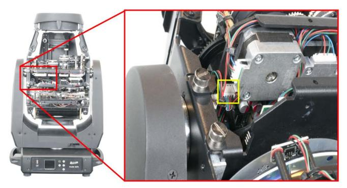
**3. Optional**. This step may be performed to help improve access to the gobo wheel module. On the prism module, find the 4-pin connector (denoted by the yellow box, above right) that is located behind the left-most electric motor, just beside the thumb screw on the left hand side of the prism module. Disconnect this connector.
