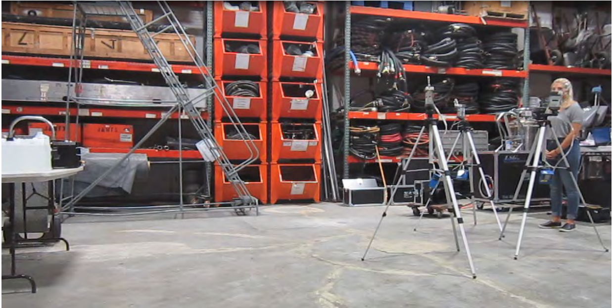
Figure 1. Configuration for calibration factor procedure, consisting of the tripod assemblies with sampling pumps, OVS tubes, and aerosol monitors.
