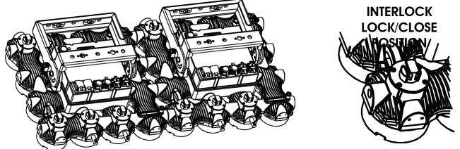
4. Repeat steps 1-3 for as needed for each horizontally/vertically connected panel.
