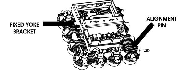
2. UNLOCK/OPEN interlocks on panel by pulling up and holding lock while turning 45 degrees to 9/3 o'clock position. Release lock so it sits completely into position. **MAKE SURE EACH INTERLOCK IS COMPLETELY IN THE 9/3 O'CLOCK UNLOCK/OPEN POSITION!**
