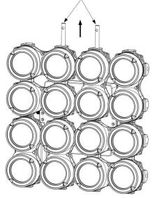
3. Insert (2x) Vertical Fixture Latches into their respective connection receptacles in the Rigging Bar
