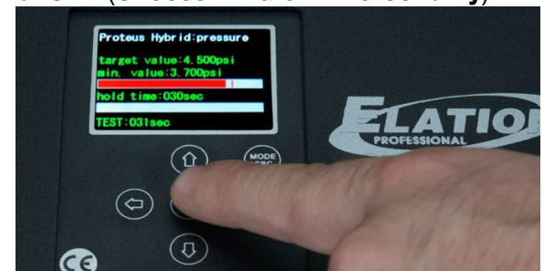
14. To enter the serial number, use ↑↓ arrows to change numbers, and use ←→ arrows to move cursor, then press <Enter> ↵ to begin the test. To bypass the input SN# altogether, just push <Enter> ↵ again.
