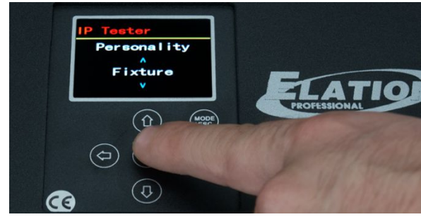
8. Select Fixture (use ←, → arrows to toggle through available fixtures) and press <Enter> ↵.
